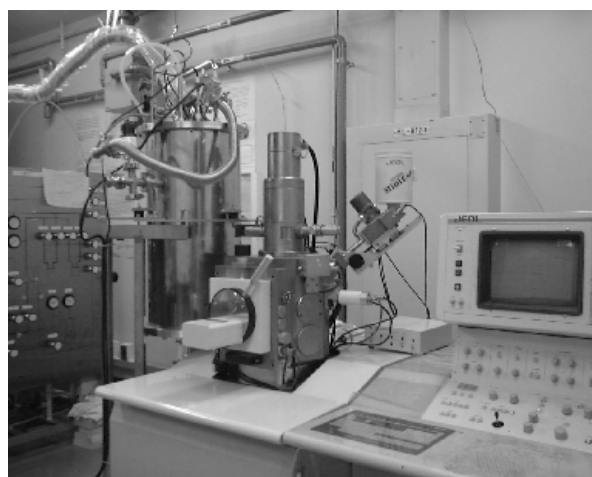
Fig. 1 SEM- microcalorimeter EDS system. This EDS system is based on the dilution refrigerator that can cool the x-ray detector below 100 mK, and has a "snout" to minimize the distance between the TES on the cold stage and sample, similar to that in a conventional semiconductor EDS system.
